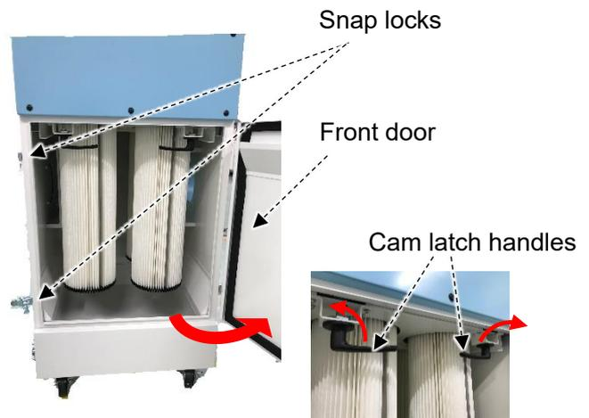
3. Pull the handle forward and remove the primary filter with its mounting plate.
