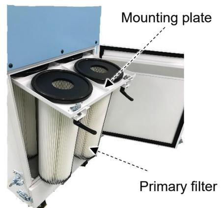
4. Remove the primary filter and attach a new primary filter.
