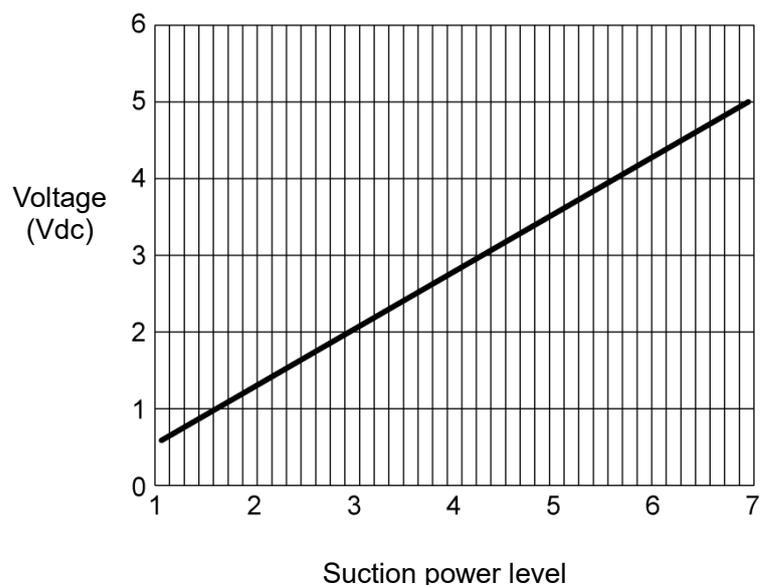
Allow for an error of  $\pm 4\%$  when setting voltage. Specifically, apply the midpoint of the voltage range for each level.
